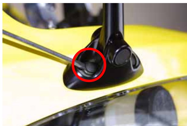
Figure 1: black plastic covers removal.
