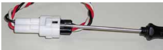
Figure 20: How to unplug a connector
