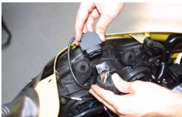
Figure 26: Wiring installation – particular of the AMP connector
