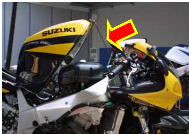
Figure 11: Uplifting the gas tank
