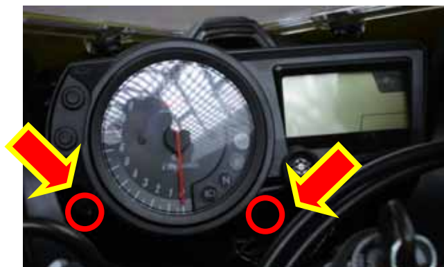
Figure 14: Position of the stock dash front screws.
