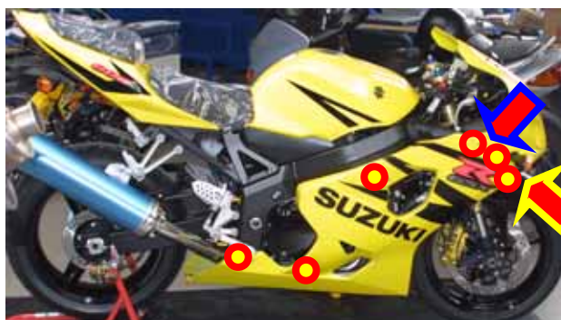
Figure 4: Right lateral fairing – screws/pins location
