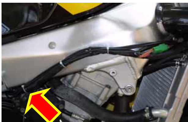
Figure 25: Wiring installation – run the wiring along the chassis
