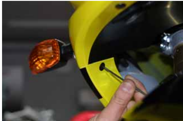
Figure 6: Unlocking the central clip of the plastic pin.
